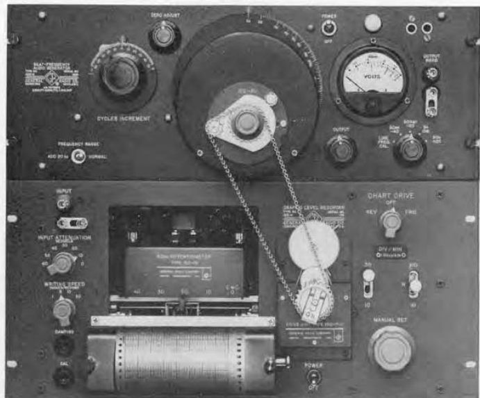
Figure 9. View of the Graphic Level Recorder coupled to drive the Beat-Frequency Audio Generator for automatic recordings of amplitude vs. frequency.
